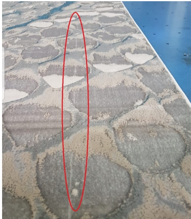
Figure 4. Photographic view of abrage failure
