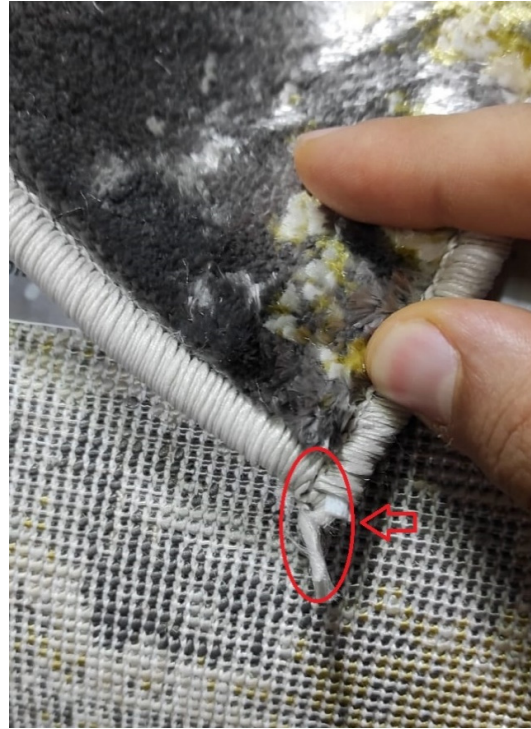
Figure 3. Photographic view of corner burning failure [19]
