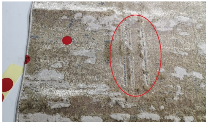
Figure 2. Photographic view of scrape failure [19]
