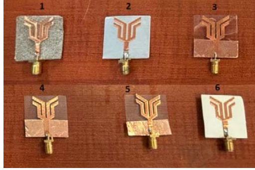
Figure 4. Photographs of fabricated Tulip-shaped microstrip antennas.
