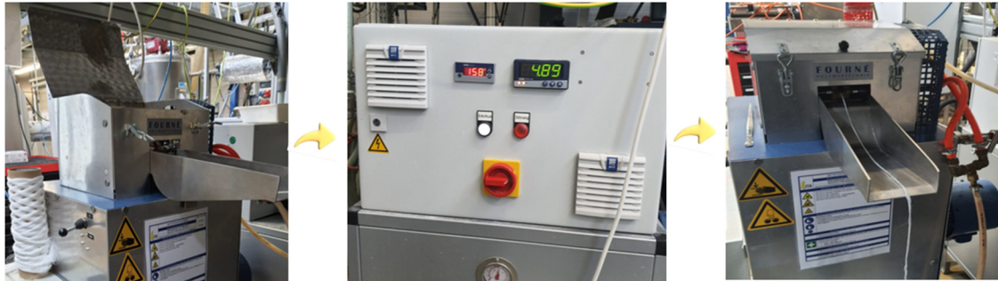
Figure 1. Imparting crimp to aerogel fibers
