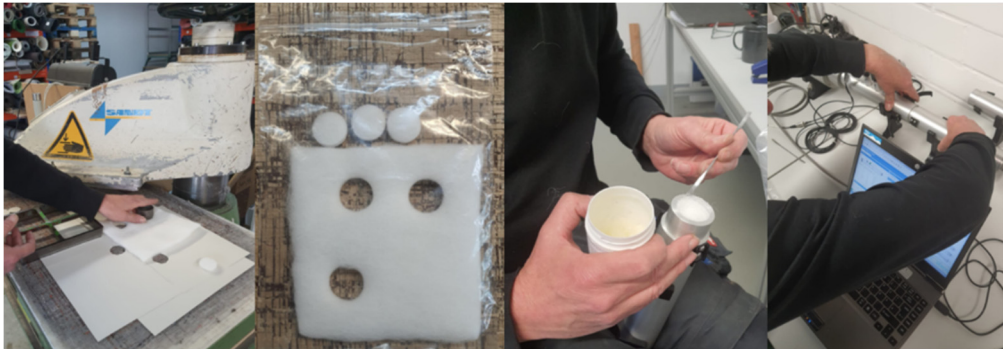
Figure 5. Preparation of samples for acoustic measurement
