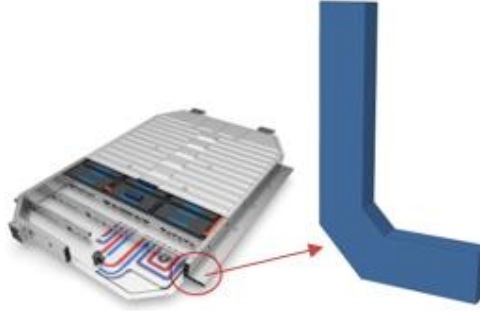
Figure 1. Battery pack housing profile of electric vehicle three-dimensional representation
