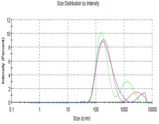
**Figure 2b.** The particle size of E7 organo-modified finishing chemical (worst softness property) (recipe 7). The particle size of E7 organo-modified was 227.9 nm (86.6 %) and solution was cloudy (Figure 2b).
