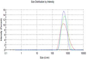
**Figure 3b.** The particle size of E9 amino-functional finishing chemical (worst softness property) (recipe 9). The particle size of E9 amino-functional was 684.2 nm (100 %), more than 1000nm, and solution was cloudy (Figure 3b).
