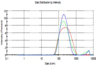
**Figure 2a.** The particle size of E1 organo-modified finishing chemical (the best softness property) (recipe 1). The particle size of E1 organo-modified was 286.3 nm (100 %) and the solution was cloudy (Figure 2a).
