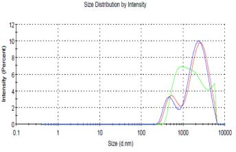
**Figure 3a.** The particle size of E8 amino-functional finishing chemical (the best softness property) (recipe 8). The particle size of E8 amino-functional was 2601 nm (81%) and solution was cloudy (Figure 3a).
