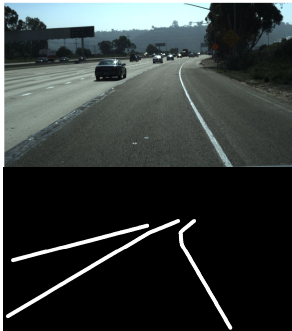
Figure 2. The 20th frame of a video clip from the TuSimple training dataset and its corresponding mask image where lane values are adjusted to 255 for clarity.
