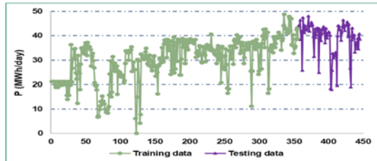
Figure 8. The training and testing data clouds of the gas generator daily total energy generation ( P )
