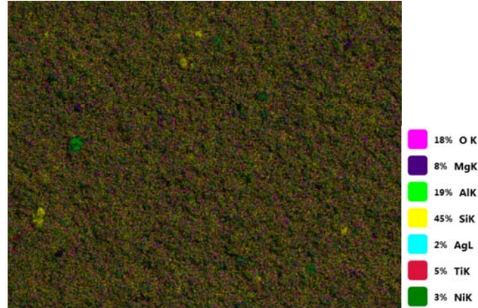
Figure 7. SEM mapping result of Ag-Ni-TiO 2 /Cordierite catalyst
