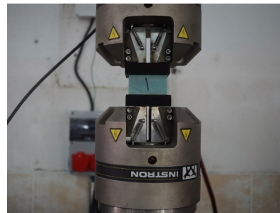
Figure 3. Compression test setup of the PVC foam core material
